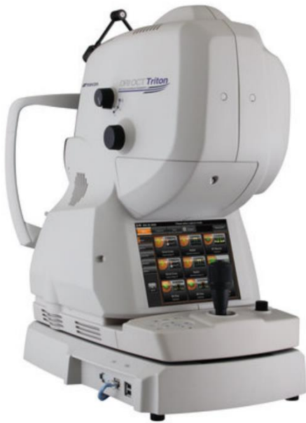
Figure 2. OCT Angiography Imaging System – DRI OCT Triton Swept Source OCT. (88)
