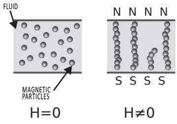
The impact of magnetic field on the ferrofluid
