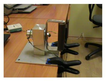
**Figure 1.** Testing station for assessment of the range of motion – goniometer
