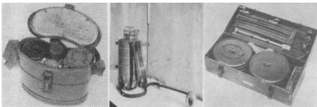
Figure 11: 23 A Heavy machine gun/mortar decontamination pack. Back pack type decontamination unit and an individual vehicle stored pack.
