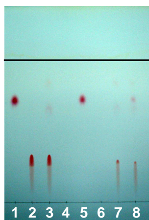
Figure 103. Photograph of the silica gel TLC plate used to demonstrate the presence of FA at the periphery of QDs. The samples were loaded on the bottom part of the plate, eluted using a 3:1:1 (v/v/v) n -butanol/acetic acid/water, and revealed with nihydriin. The 8 lanes correspond to (1) commercial glutamic acid, (2) commercial PEGamine, (3) PEGamine after acid hydrolysis, (4) commercial folic acid, (5) folic acid after acid hydrolysis, (6) ZnS:Mn/ZnS@MPA QDs after acid hydrolysis, (7) PEGamine-functionalized ZnS:Mn/ZnS QDs after acid hydrolysis, and (8) folic acid-functionalized ZnS:Mn/ZnS QDs after acid hydrolysis.
